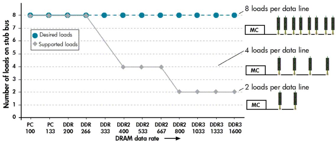
The parallel interface for each DRAM-II channel requires 240 pins. Increasing the number of channels to compensate for the drop in capacity per channel was not a viable option due to increased cost and board complexity. Therefore, a new serial memory interface with a lower pin count and point-to-point connections was needed to reach the higher memory bandwidth required by future generations of servers.
