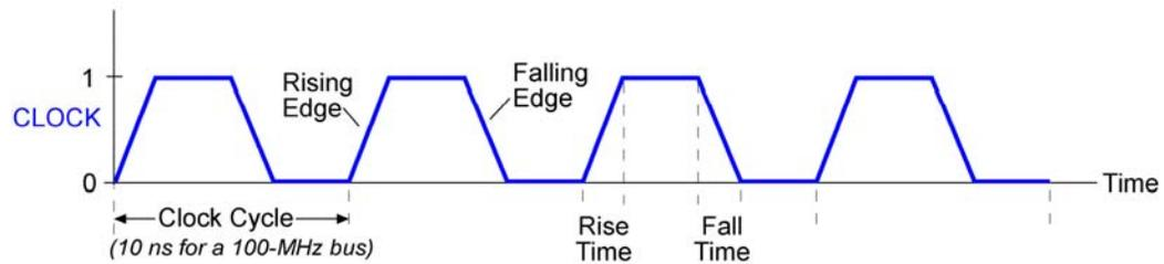
*The clock cycle time is measured in nanoseconds (ns,  $1 \times 10^{-9}$  second) and the clock frequency is measured in megahertz (MHz, millions of cycles per second). The clock frequency is the reciprocal of the clock cycle time. For example, if the clock cycle is 10 ns then the clock frequency is  $1/(0.000000010)=100$  MHz.*
