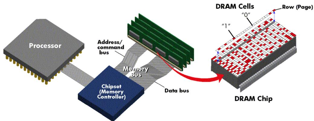
The memory subsystem operates at the memory bus speed. Typically, a DRAM cell is accessed when the memory controller sends electronic address signals that specify the row address and column address of the target cell. The memory controller sends these signals to the DRAM chip by way of the memory bus. The memory bus consists of two sub-buses: the address/command bus and the data bus.
